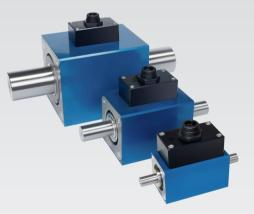
Up to 100 N·m, no bearing friction on measuring side Non-contact signal transmission Measuring amplifier is not necessary Evaluation on PC, directly Maintenance-free Accuracy class 0,1
